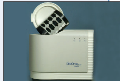
Figure 4: DenOptix laser scanner (Gendex Dental Systems, Des Plaines, Ill.), illustrating the drum on which storage phosphor plates are clipped. The drum is inserted into the scanner and the lid is closed before scanning.
