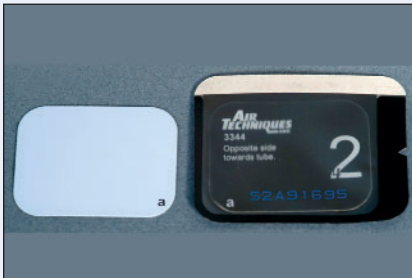
Figure 3: Storage phosphor plate (Air Techniques, Hicksville, N.Y.) illustrating the active (tube side) surface of the plate (left) and plate placed in the infection control pouch (right). The plate is oriented with the tube side against the black (opaque) side of the pouch to limit exposure of the active side of the plate to ambient light.
