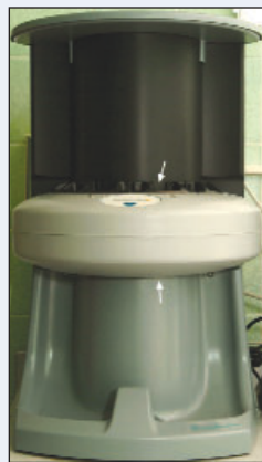
Figure 5: ScanX laser scanner (Air Techniques, Hicksville, N.Y.) Storage phosphor plates are inserted at the top of the scanner (top arrow) and ejected (bottom arrow) after scanning is complete.
