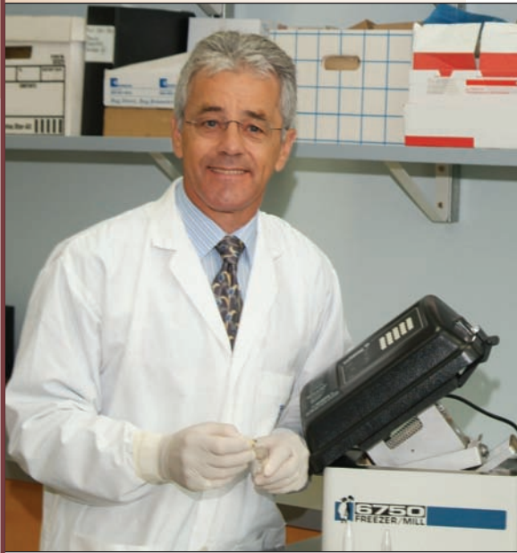
Dr. Sweet at the BOLD lab. The freezer mill shown in the photo is used to cryogenically prepare a bone sample for DNA extraction. Photo credit: Dr. Leon Woolf.
