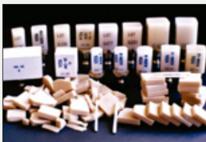
Figure 1: Numerous new ceramics with different properties are available today for computer-aided design and computer-aided manufacture (CAD/CAM). The long-term performance of these ceramics remains unknown. (Product range of Vita GmbH, Germany.)
