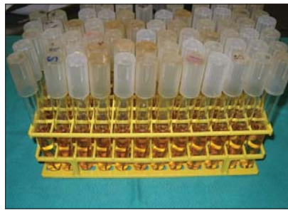
Figure 2: The instruments were placed into test tubes and stored vertically in racks in a 37°C incubator.
