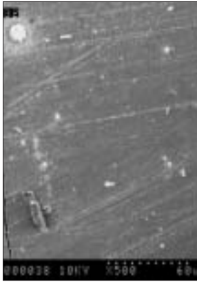
Figure 3a: Bovine tooth after enamel reduction with a diamond disk plus 3M polishing disks.
