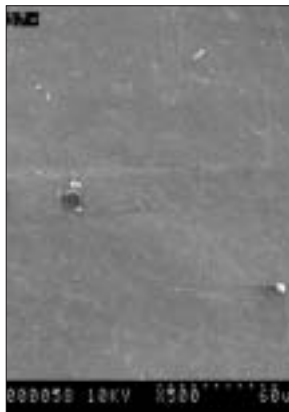
Figure 3c: Bovine tooth after enamel reduction with a diamond disk plus 3M polishing disks plus 10% maleic acid.
