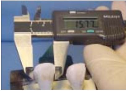
Figure 1: Digital calipers indicating measurement to 0.01 mm.
