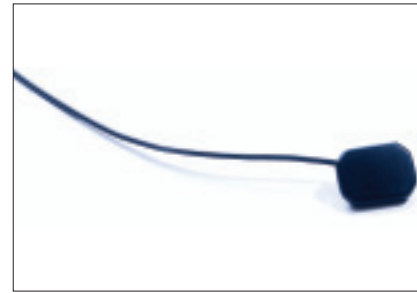
Figure 1: The sensor for the Dexis digital radiography system measures 1.5 inches \times 1.14 inches \times 0.3 inches.
